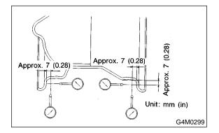
4) If rim runout exceeds specifications, remove tire from rim and check runout while attaching dial gauge to positions shown in figure.
