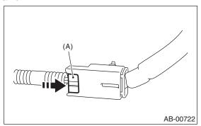
(2) With the slide lock pushed in, disconnect the connector.
