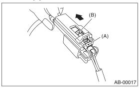
(3) With the slide lock pulled, release the lock arm (return to original position) and disconnect the connector.
