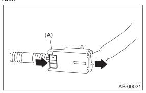
(2) With the slide lock pushed, pull it in the direction of arrow and disconnect the connector.
