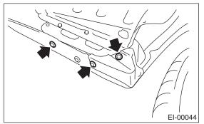
4) When removing the rear bumper beam assembly, remove the six bolts from bumper stay.
