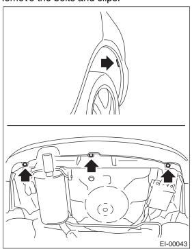
3) Remove the clips from the bumper and bracket.
