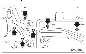
5) Loosen screws to remove motor assembly.
