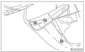
3) Turn over the mud guard and turn the socket and then remove the bulb.
