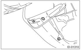
3) Turn over the mud guard, turn the socket and then remove the bulb.
