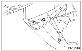
3) Remove the spring retainer then detach the fog light bulb.
