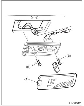
3) Disconnect the harness connectors and remove the luggage room light.
