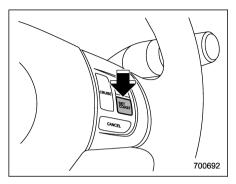
3. Push the "SET/COAST" button and release it. Then release the accelerator pedal.
