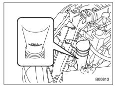
Remove the washer tank filler cap, then check the fluid level indicated by the level gauge (attached to the inside of the cap). If the level is near the "Low" mark, add fluid until it reaches the "Hi" level on the
