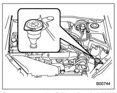
If you spray washer fluid on the windshield but the supply of washer fluid appears to diminish, check the level of washer fluid in the tank.
