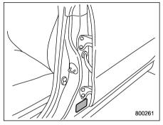
The certification label attached to the driver's side dooriamb shows GVWR (Gross Vehicle Weight Rating) and GAWR (Gross Axle Weight Rating).
