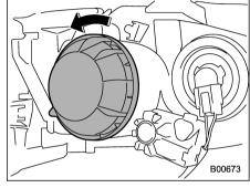
3. Remove the bulb cover, by turning it counterclockwise.
