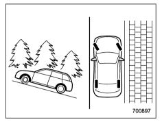
When the vehicle is facing uphill, the front wheels should be turned away from the curb.
