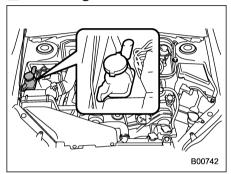
The power steering fluid expands greatly as its temperature rises; the fluid level differs according to fluid temperature. Therefore, the reservoir tank has two different checking ranges for hot and cold fluids.
