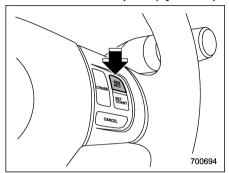
Push the "RFS/ACC" button and hold it until the vehicle reaches the desired speed. Then, release the button. The vehicle speed at that moment will be memorized and treated as the new set speed.
