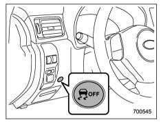
Pressing the switch to deactivate the Vehicle Dynamics Control system can facilitate the following operations:
