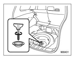
16. Store the flat tire in the spare tire compartment. Put in the spacer and tighten the attaching bolt firmly.
