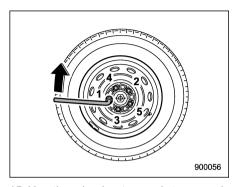
15. Use the wheel nut wrench to securely tighten the wheel nuts to the specified torque, following the tightening order in the illustration.
