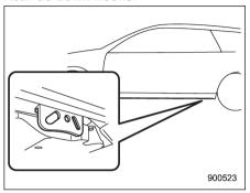
The rear tie-down hooks are located near each of the jack-up reinforcements.
