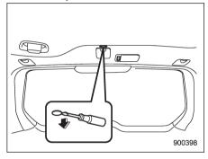
1. Remove the plug on the roof trim of the cargo area by inserting the end of the flathead screwdriver between the roof and plug and prying it off.
