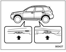
9. Place the jack under the side sill at the front or rear jack-up point closest to the flat tire.
