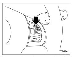
To resume the cruise control after it has been temporarily canceled and with vehicle speed of approximately 20 mph (32 km/h) or more, push the "RES/ACC" button to return to the original cruising speed automatically.
