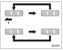
Models equipped with unidirectional tires
