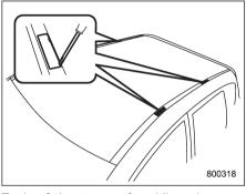
Each of the two roof moldings has two mounting points for crossbars. Each mounting point is fitted with a cover. Use a screwdriver to remove the covers. When installing the crossbars on the roof molding, follow the manufacturer's instructions.
