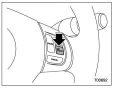
Push the "SFT/COAST" button and hold it until the vehicle reaches the desired speed. Then, release the button. The vehicle speed at that moment will be memorized and treated as the new set speed.
