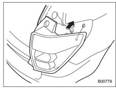
6. Put the rear combination light assembly into place while aligning the clip with the guide on the vehicle.
