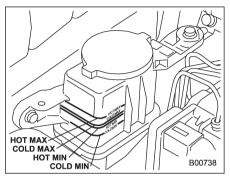
2. Check the fluid level of the reservoir tank.
