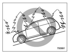
The Hill start assist system does not operate when the vehicle is facing down-hill. And the Hill start assist system may not operate on slight grades.
