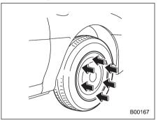
Align the valve with the valve hole in the cover, then fit the cover on the wheel by tapping your hand evenly around the circumference of the cover
