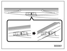
2. Turn the wiper blade assembly counterclockwise.
