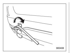
4. Tighten the towing hook securely using a wheel nut wrench.
