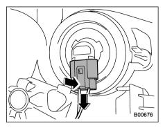
2. Disconnect the electrical connector from the bulb
