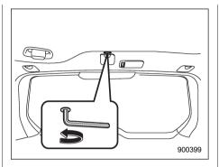
2. Insert a hex-head wrench in the end of the motor shaft.
