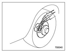
The front disc brake and the rear disc brake have audible wear indicators on the brake pads. If the brake pads wear close to their service limit, the wear indicator makes a very audible scraping noise when the brake pedal is applied.
