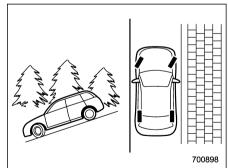
When the vehicle is facing downhill, the front wheels should be turned into the curb.
