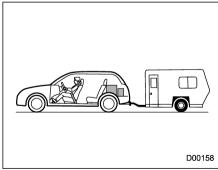
Vehicle capacity weight of the vehicle is 900 lbs (408 kg), which is indicated on the vehicle placard
