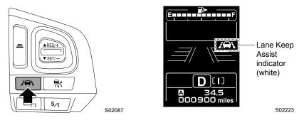
Press the (Lane Keep Assist) switch once again to turn it off, and " (Lane Keep Assist indicator) is turned off on the EyeSight display area.
