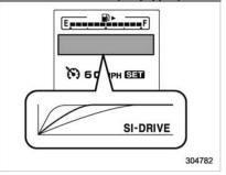
This screen indicates the current SI-DRIVE mode with its throttle angle.
