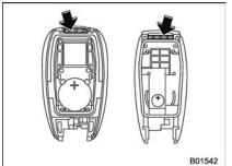
5. Attach the cover to the access key by fitting the projections and recesses together.
