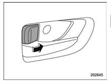
2. Rotate the lock lever forward.
