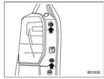
1. Using a Phillips screwdriver, remove the upper and lower screws that secure the rear combination light assembly.
