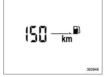
The driving range indicates the distance that can be driven taking into account the amount of fuel remaining in the tank and
