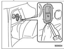
1. Release the fitting on the left side rear seat release latch.
