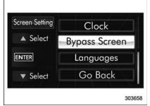
2. Operate the "▲" or "▼" switch to select the "Bypass Screen" item. Then push the ENTER button.
