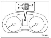
Select lever/gear position indicator (type A)
