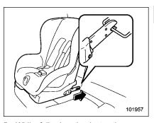
5. While following the instructions supplied by the child restraint system manufacturer, connect the lower hooks onto the lower anchorages located at "Q" marks on the bottom of the rear seatback. When the hooks are connected, make sure the adjacent seatbelts are not caught.
