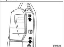
7. Tighten the upper and lower screws.
