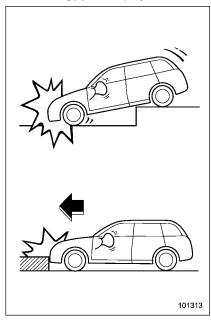
Only the driver's SRS frontal airbag or both driver's and front passenger's SRS frontal airbags may be activated when the vehicle sustains a hard impact in the undercarriage area from the road surface (such as when the vehicle plunges into a deep ditch, is severely impacted or knocked hard against an obstacle on the road such as a curb).
