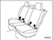
The lower anchorages (bars) are provided for installing a child restraint system only on the rear seat window-side seating positions. For each window-side seating position, two lower anchorages are provided
