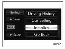
3. After the selection screen is displayed, operate the "▲" or "▼" switch to show the "Initialize" item. Then, push the REE button.
