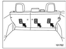
The tether anchorages (upper anchorages) are provided at the locations shown in the above illustration. For details, refer to "Top tether anchorages" \$\tilde{\Cappa} 1-\$ 40.
