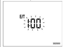
The journey time indication flashes each time a complete hour has elapsed. If the display is giving a reading other than the journey time, the display switches to the journey time, flashes for 5 seconds, and returns to its original reading each time a complete hour has elapsed.
