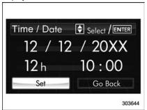
5. After entering the date and time, select "Set" by operating the "V" switch and confirm the setting by pushing the ENTER button.
