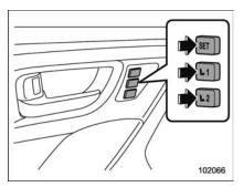
2. While pressing the "SET" button, press and hold the desired button "1" or "2".
