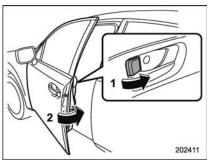
Locking using lock lever
