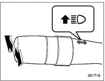
To change from low beam to high beam, push the turn signal lever forward. When the headlights are on high beam, the high beam indicator light "ED" on the combination meter is also on.
