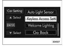
2. Operate the "▲" or "▼" switch to select the "Keyless Access Setting" item. Then push the ⊞ button.
