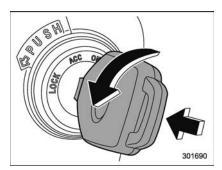
The key can be turned from the "ACC" to "LOCK" position only when the select lever is in the "P" position (CVT models) and the key is pushed in while turning it (all models).
