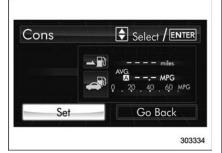
5. Select "Set" by operating the "▼" switch, and confirm the setting by pushing the ENTER button.
