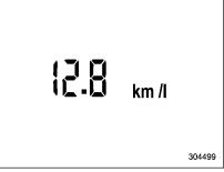
This display shows the average rate of fuel consumption since the trip meter was last reset.
