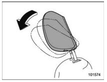
The angle of the head restraint can be adjusted in several steps. While maintaining a suitable driving posture, adjust the head restraint to a position where the back of your head is as close to the head restraint as possible.
