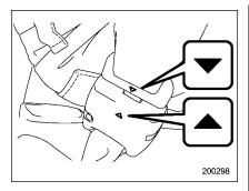
4. After fastening the seatbelt, make sure that the "V" mark on the connector (tongue) and the "A" mark on the buckle face outwards.
