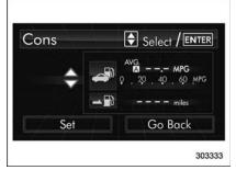
4. Select the displayed configuration by operating the "▲" or "▼" switch. Then push the ENTER button.
