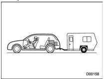
Vehicle capacity weight of the vehicle is 900 lbs (408 kg), which is indicated on the vehicle placard
