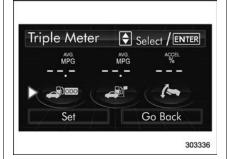
3. Select the setting location (left, center or right) by operating the " $\blacktriangledown$ " or " $\blacktriangle$ " switch. Then push the <code>misk</code> button.
