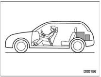
Vehicle capacity weight of the vehicle is 900 lbs (408 kg), which is indicated on the vehicle placard with the statement "The combined weight of occupants and cargo should never exceed 900 lbs or 408 ka".
