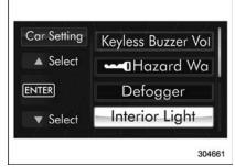
2. Operate the " $\blacktriangle$ " or " $\blacktriangledown$ " switch to select the "Interior Light" item. Then push the  $\blacksquare$  button.
