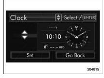
4. Select "Type A clock", "Type B clock", "Calendar" or "Off" by operating the "▼" switch. Then push the ▶ button.
