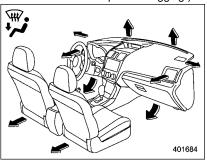
**(Heat-def):** Windshield defroster outlets, foot outlets and both side outlets of the instrument panel (Refer to "Defrosting" \$\tilde{\pi}\$4-11.)
