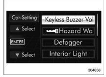
2. Operate the "▲" or "▼" switch to select the "Keyless Buzzer Volume" item. Then push the button.
