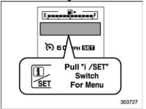
While this screen is selected, pull the "T/SET" switch to enter the menu screen.
