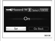
5. Select "Set" by operating the "▼" switch, and confirm the setting by pushing the receipt button.
