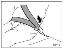
1. Push the release button of the center seatbelt buckle (on the left-hand side) to unfasten the seatbelt.
