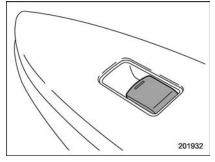
Each passenger window can be controlled by the power window switch located on the door.
