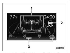
When the Vehicle Dynamics Control system has been activated: the tires remain illuminated in yellow while the Vehicle Dynamics Control System is activated.
