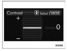
3. Select a contrast level by operating the "\Lambda" or "\textbf\" switch, and confirm the setting by pushing the ENTER button.
