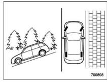
When facing downhill, the front wheels should be turned into the curb.
