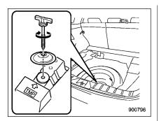
17. When storing the spare tire after repairing a flat tire, be sure to place the spacer in the manner shown in the illustration, and then tighten the bolt in the rear side of the bracket.
