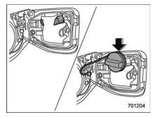
3. Set the fuel filler cap on the cap holder inside the fuel filler lid
