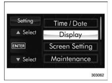
3. After the selection screen is displayed, operate the "A" or "V" switch to show the "Display" item. Then, push the ENTER button.
