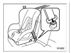
12. To remove the child restraint system, press the release button on the seatbelt buckle and allow the belt to retract completely. The belt will return to the FIR mode.
