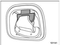
3. Allow the retractor to roll up the belt.
