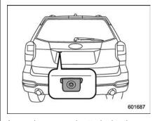
A rear view camera is attached to the rear gate. When the ignition switch is "ON" and the shift lever (MT models) or select lever (CVT models) is set to "R", the rear view camera automatically displays the rear view image behind the vehicle on the monitor of the navigation system or the audio display.
