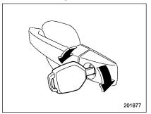
To lock the driver's door from the outside with the key, turn the key toward the front.
