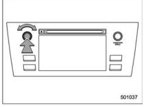
Press the power/VOLUME knob to turn the audio/visual system on and off. When the system turns on, the mode that was in use the last time the system was turned off will be displayed. Press and hold the knob to turn the display off.
