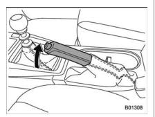
Check the parking brake stroke according to the maintenance schedule in the "Warranty and Maintenance Booklet". When the parking brake is properly adjusted, braking power is fully applied by pulling the lever up 7 to 8 notches gently but firmly (approximately 45 lbf [200 N, 20.4 kgf]). If the parking brake lever stroke is not within the specified range, have the brake system checked and adjusted at your SUBARU dealer.
