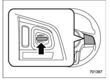
To resume the cruise control after it has been temporarily canceled and with vehicle speed of approximately 20 mph (30 km/h) or more, press the "RES/SET" switch to the "RFS" side to return to the original cruising speed automatically.
