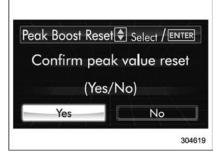
2. Select "Yes" by operating the "\nstacks" switch, and confirm the resetting by pushing the \text{ entre} button.
