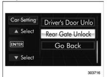
2. Operate the "▲" or "▼" switch to select the "Rear Gate Unlock" item. Then push the button.
