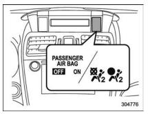
ON / St. Front passenger's frontal airbag ON indicator
