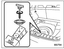
16. Store the flat tire in the spare tire compartment. Be sure to place the spacer in the manner shown in the illustration, and then tighten the bolt in the front side of the bracket.
