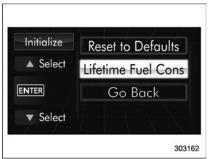
2. Operate the "▲" or "▼" switch to select the "Lifetime Fuel Consumption Resetting" item. Then push the with button.
