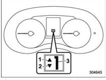
Select lever/gear position indicator (type B)
