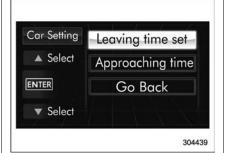
3. Select the "Leaving time set" by operating the "▲" or "▼" switch, and then push the RIER button.
