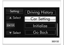
3. After the selection screen is displayed, operate the "▲" or "♥" switch to show the "Car Setting" item. Then, push the button.
