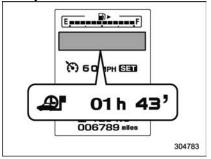
This screen displays the journey time (the time that has elapsed since the ignition switch was turned to the "ON" position).
