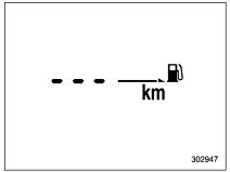
If the driving range is shown as "---". there is only a tiny amount of fuel left in the tank. You must refuel the vehicle immediately.
