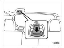
Rear center seatbelt is stowed in the recess of the ceiling above the cargo area.
