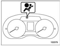
SRS airbag system warning light (type A)
