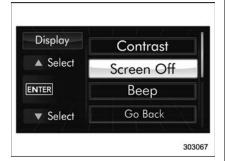
2. Operate the "\( \bigs\_{\text{"}}\)" or "\( \bigs\_{\text{"}}\)" switch to select the "Screen Off" item. Then push the (ENTER) button.
