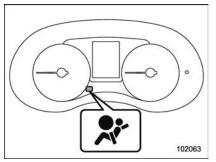
SRS airbag system warning light (type B)
