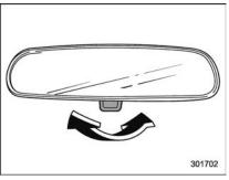
The inside mirror has a day and night position. Pull the tab at the bottom of the mirror toward you for the night position. Push it away for the day position. The night position reduces glare from headliahts.
