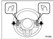
To upshift to the next higher gear position, pull the shift paddle that has "+" indicated on it. To downshift to the next lower gear position, pull the shift paddle that has "-" indicated on it.
