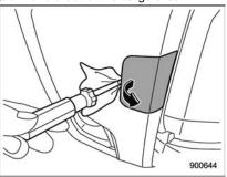
2. Cover the tip of a flat-head screwdriver with vinvl tape or cloth so that it will not scratch the bumper. Insert the flat-head screwdriver into the cutout of the cover and prv open the cover.
