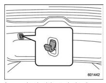
A convenient hook is attached to the rear gate trim. When the rear gate is open, you can hang a candle lantern, wet suit, etc. on the hook.
