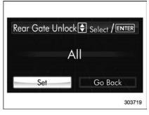
5. Select "Set" by operating the "▼" switch, and confirm the setting by pushing the ■■■ button.
