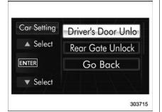
2. Operate the "▲" or "▼" switch to select the "Driver's Door Unlock" item. Then push the button.
