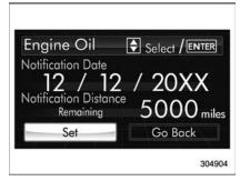
5. Select "Set" by operating the "▲" or "▼" switch and confirm the setting by
