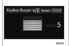
3. Select a volume level by operating the "▲" or "▼" switch, and confirm the setting by pushing the button.
