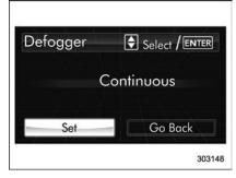
5. Select "Set" by operating the "▼" switch, and confirm the setting by pushing the will button.
