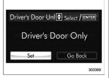
5. Select "Set" by operating the "▼" switch, and confirm the setting by pushing the wise button.
