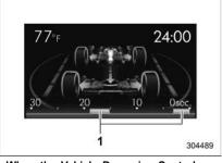
When the Vehicle Dynamics Control system is being activated: the tires illuminate in yellow.
