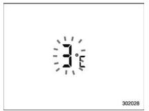
When the outside temperature drops to  $37^{\circ}F$  ( $3^{\circ}C$ ) or lower, the temperature indication flashes to show that the road surface may be frozen.
