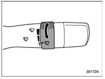
When the wiper switch is in the "\subsetexts" position, turn the dial to adjust the operating interval of the wiper. The operating interval can be adjusted in several steps from the shortest interval to the longest.
