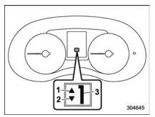
Select lever/gear position indicator (type B)
