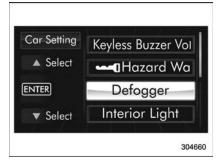
2. Operate the " $\blacktriangle$ " or " $\blacktriangledown$ " switch to select the "Defogger" item. Then push the
