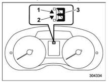
Select lever/gear position indicator (type A)
