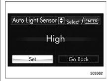
5. Select "Set" by operating the "▼" switch, and confirm the setting by pushing the ▶ button.
