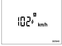
This display shows the average vehicle speed since the trip meter was last reset.
