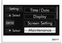
3. After the selection screen is displayed, operate the "\( \Lambda \)" or "\( \nabla \)" switch to show the "Maintenance" item. Then, push the ENTER button.
