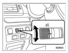
The illumination brightness of the instrument panel dims under the following conditions.
