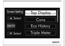
2. Operate the "▲" or "▼" switch to select the "Top Display" item. Then push the ™™ button.
