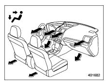
(Bi-level): Instrument panel outlets and foot outlets
