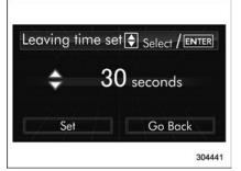
5. Select the preferred setting by operating the "\( \Lambda \)" or "\( \nstacksigma \)" switch, and then push the ENDER button.
