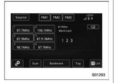
1. Touch the "Tag" key in the control screen while receiving HD Radio, the tag setting screen will be displayed.
