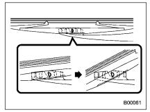
2. Turn the wiper blade assembly counterclockwise.
