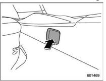
1. Insert the protrusion located on the right end of the sleeve into the recess of the retainer.
