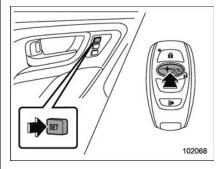
2. While holding the access key and pressing the "SET" button, press the "a" button of the access key.
