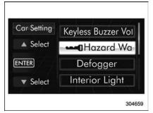
2. Operate the "▲" or "▼" switch to select the "Hazard Warning Flasher" item. Then push the button.
