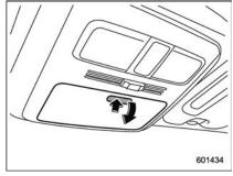
To open the console, push on the console lid lightly. The lid will automatically open.
