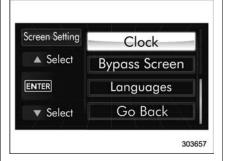
2. Operate the "▲" or "▼" switch to select the "Clock" item. Then push the button.
