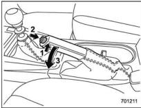
To release the parking brake, perform the following procedure.
