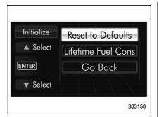
2. Operate the "▲" or "▼" switch to select the "Reset to Defaults" item. Then push the ■■■ button.
