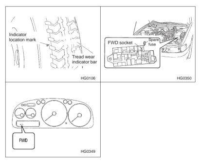
• (If your vehicle is AWD with automatic transmission) Before driving your vehicle with the temporary spare tire, put a spare fuse inside the FWD connector in the main fuse box located in the engine compartment and confirm that the Front-wheel drive warning light comes on. The all wheel drive capability of the vehicle has now deactivated. Af-
