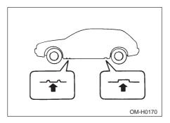
9. Insert the jack handle into the jackscrew, and turn the handle clockwise until the tire clears the ground. Do not raise the vehicle higher than necessary.
