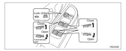
All door windows can be controlled by the power window switch cluster at the driver side door.
