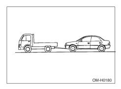
We do not recommend this method of towing. Use this method only when towing service by a SUBARU dealer or a commercial towing service is not available.
