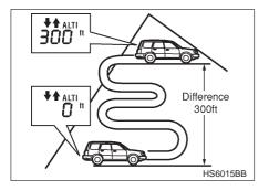
The altimeter indicates the relative elevation.
