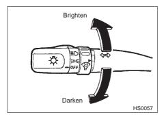
When the lighting switch is in the "うのだ" or "置O" position, you can adjust brightness of the instrument panel illumination for better visibility. To brighten, turn the control dial counterclockwise.
