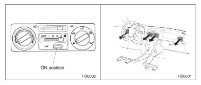
For cooling and dehumidification of the passenger compartment, air flows through the instrument panel outlets:
