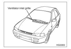
Always keep the front ventilator inlet grille free of snow, leaves, or other obstructions to ensure efficient heating and defrosting. Since the condenser is located in front of the radiator, this area should be kept clean
