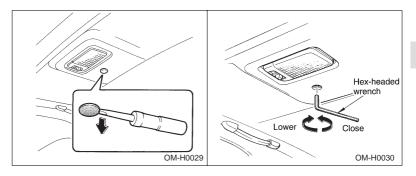
If the sunroof can not be closed with the sunroof switch, you can close the roof manually.
