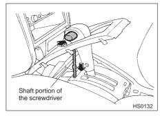
6. Draw the shaft portion of the screwdriver from the grip and then insert the shaft into the hole.
