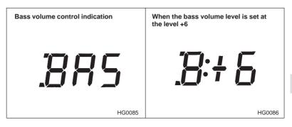
Select the Bass control mode by pressing the "T/B" button. In the bass control mode, the display shows the indication as shown.
