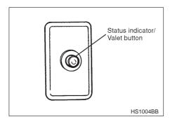
The Status Indicator is a high intensity warning light, located on the dash to the left of the steering wheel. The Status Indicator displays a visual indication of the security system's status while creating a powerful theft deterrent.
