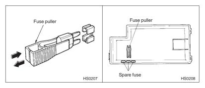
4. Pull out the fuse with the fuse puller. The fuse puller is stored in the main fuse box cover in the engine compartment.
