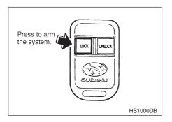
To arm the system, close all doors, then press the "LOCK" button. The siren will "chirp" twice and the parking lights will flash twice, indicating the system is armed.
