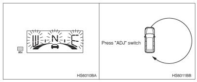
1) Press the "ADJ" switch for the compass setting mode.
