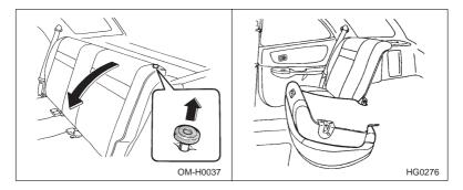
Unlock the seatback by pulling the release knob and fold it down.
