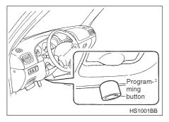
The Programming Button is located under the driver's side dash beneath the diagnostic connector.
