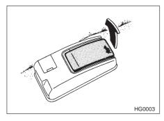
Pull the trunk lid release lever upward.
