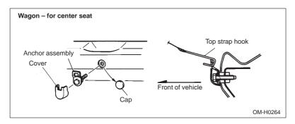
2. Remove the cover of the anchor installation point.
