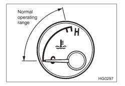
The temperature gauge shows engine coolant temperature when the ignition switch is in the "ON" position.
