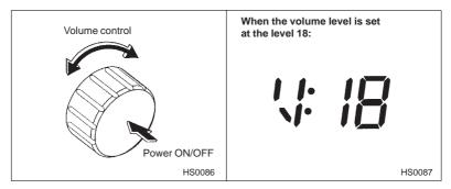
The same knob is used for both power (on/off) and volume control. The radio is turned on and off by pushing the knob and the volume is controlled by turning the knob.
