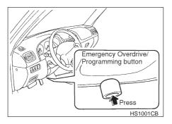
If your remote transmitter fails to operate, the system can be disarmed using the Emergency Override/Programming button. Follow the procedure below:
