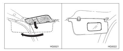
To block out glare, swing down the visors. To use the sun visor at a side window, swing it down and move it sideways.
