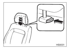
To raise the head restraint, pull it up. To lower it, push the head restraint down while depressing the release button on the top of the seatback.
