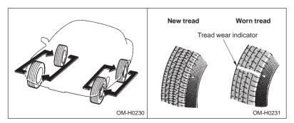
A tire should be replaced when the tread wear indicator appears as a solid band across the tread. The indicators appear when the remaining tread has been worn to 0.063 in (1.6 mm) or less.
