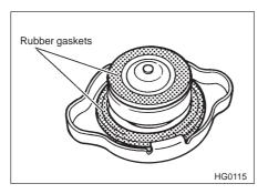
4. Put the radiator cap back on and tighten firmly. At this time, make sure that the rubber gaskets in the radiator cap is correctly in place.
