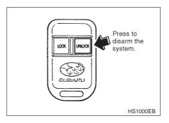
To disarm the system, press and release the "UNLOCK" button. The siren will chirp and parking lights will flash **once**. The driver's door will unlock at this time, and the vehicle interior (dome) light will turn on for 60 seconds, or until the vehicle is started.
