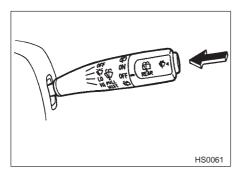
To wash the windshield, push the washer button at the end of the wiper control lever. The washer fluid sprays until you release the washer button. The wipers operate while you push the button.
