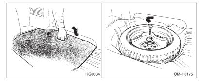
The spare tire is stored under the floor of the trunk or the luggage compartment. To remove the spare tire, first remove the spare tire cover, turn the attaching bolt counterclockwise, then take the spare tire out.
