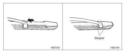
6. Install the wiper blade assembly to the wiper arm. Make sure that it locks in place.
