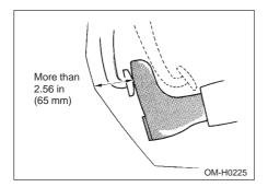
– CONTINUED – 10-37 Depress the pedal with a force of approximately 294 N (66 lb., 30 kg) and measure the distance between the upper surface of the pedal pad and the floor.
