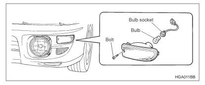
1. Remove the bolt securing the front turn signal light assembly.
