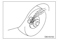
The front disc brake has an audible wear indicator on the brake pads. For RS models, the right side rear disc brake also has a audible wear indicator. If the brake pads wear close to their service limit, the wear indicator makes a very audible scraping noise when the brake pedal is applied.
