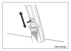
The shoulder belt anchor height should be adjusted to the position best for you. To adjust the anchor height, pull the release knob and move the anchor to the desired position so that the shoulder belt passes over the middle of the shoulder without touching the neck.
