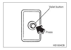
Valet Mode prevents the security system from arming, yet allows all keyless entry and convenience features to function normally.
