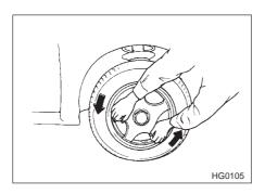
Grasp the wheel cover with both hands by the spokes and twist sharply in a **counterclockwise** direction until you feel the detent release. Now the wheel cover is free from the retention ring.
