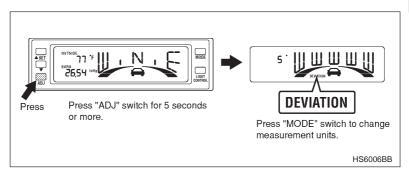
1. Turn on the ignition switch to the "ACC" position and the display shows the default English measurement units.
