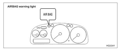
A diagnostic system continually monitors the readiness of the SRS AIR-BAG while the vehicle is being driven. The SRS AIRBAG warning light will show normal system operation by lighting for about 6 seconds when the ignition key is turned to the "ON" position.
