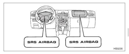
The driver's side SRS AIRBAG is stored in the center portion of the steering wheel. The passenger's side SRS AIRBAG is stored near the top of the dashboard under the cover marked "SRS AIRBAG".
