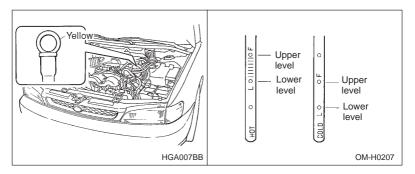
4. Pull out the dipstick and check the fluid level on the gauge. If it is below the lower level on the "HOT" range, add the recommended automatic transmission fluid up to the upper level.
