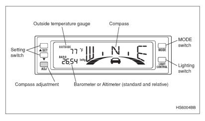
• The display operates when the ignition switch is in the "ACC" or "ON" position.
