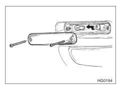
1. Remove the front turn signal light assembly mounting screws using the phillips screwdriver.
