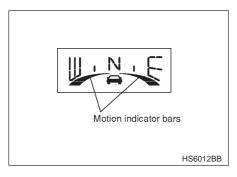
1. 1.8 mile/h (2.8 km/h) of vehicle speed  $\ldots$  1 second interval bar motion.
