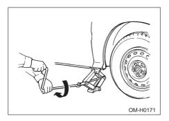
10. Remove the wheel nuts and the flat tire.
