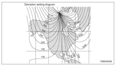
Depending on your location, the following adjustment is required due to the difference between magnetic and geographic North. Refer to the map shown above for the setting most appropriate for your location.
