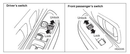
All doors and the rear gate can be locked and unlocked by the power door locking switches at the driver's side and the front passenger's side doors.
