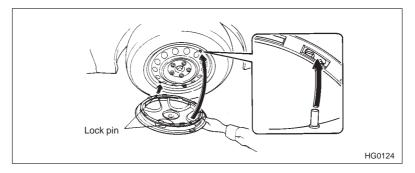
2. Grasp the wheel cover with both hands by the spokes and twist sharply in a **clockwise** direction until you feel the detent locking. After twisting the wheel cover, make sure the wheel cover is locked securely by lightly turning the wheel cover right and left.
