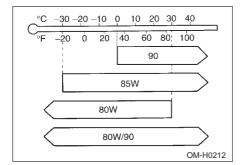
SAE viscosity No. and Applicable Temperature
