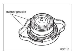
3. After refilling the reserve tank and the radiator, reinstall the caps and check that the rubber gasket inside the radiator cap is in the proper position.
