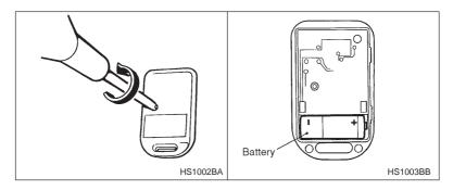
1. Remove the phillips screw on the back of the remote transmitter case. Use a small coin to separate the case halves and expose the battery.
