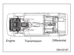
Inspect the following for oil leaks:
