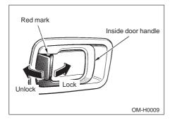
To lock the door from the inside, press the end of the lock lever down. To unlock the door from the inside, pull the front end of the lock lever.
