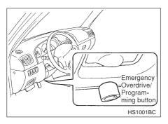
The Emergency Override/Programming button is used to disarm the alarm system in case of a lost or broken transmitter. It is also used in conjunction with the transmitter and vehicle ignition to program additional transmitters.
