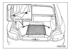
The luggage compartment is equipped with four anchorage eyelets for securing luggage with a luggage net or ropes.
