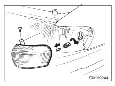
1. Remove the parking light assembly mounting screw located at the top of the headlight assembly using the phillips screwdriver.
