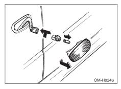
1. Pull the left side of the turn signal light assembly while moving it forward in relation to the vehicle.
