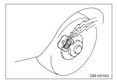
The disc brake pad wear warning indicators on the disc brakes give a warning noise when the brake pads are worn.
