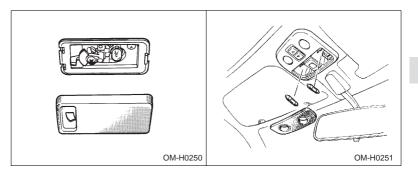
1. Remove the lens by prying the edge of the lens with a regular screwdriver.
