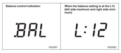
Select the Balance control mode by pressing the "T/B" button. In the balance control mode, the display shows the indication as shown.
