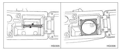
The front passenger's cup holder is built in the center console. To use the cup holder, open the lid of the console and open the holder. When not in use, fold the holder and close the lid.
