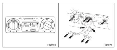
This setting allows you to direct air of different temperatures from the instrument panel and outlets. The air from the foot outlets is slightly
