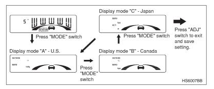
3. Change the measurement units by pressing the "MODE" switch until the proper mode appears.
