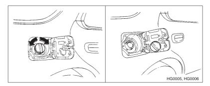
To take off the fuel filler cap, turn it slowly counterclockwise and remove the cap. While refueling, hang the cap on the cap holder inside the fuel lid.
