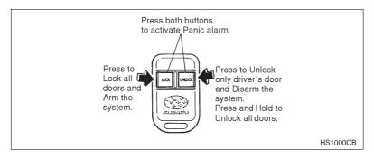
The security system can be programmed to operate with one to four remote transmitters. Each transmitter is powered by an internal 12-volt alkaline battery.
