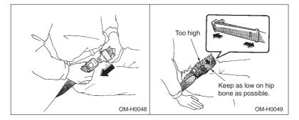
1. Sit well back in the seat and pick up the tongue plate marked "CEN-TER". Be careful not to twist the belt.
