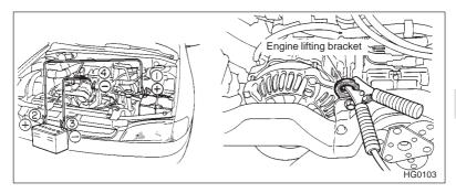
1 Connect one jumper cable to the positive (+) terminal on the discharged battery.
