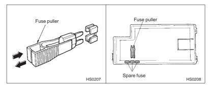
5. Pull out the fuse with the fuse puller provided in the main fuse box cover.
