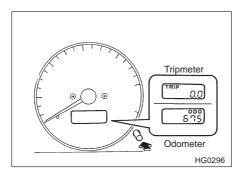
This meter displays the odometer and trip meter when the ignition switch is in the "ON" position.
