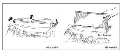
1. Remove the bolt securing the rear air cleaner element case.
