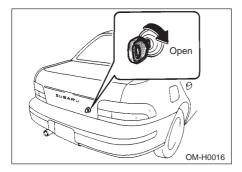
To open the trunk lid from outside, insert the key in the keyhole and turn it clockwise. To close the trunk lid, lightly press the trunk lid down until the latch engages.
