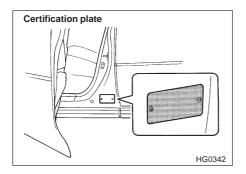
The certification plate attached to the driver's side door jamb shows GVWR (Gross Vehicle Weight Rating) and GAWR (Gross Axle Weight
