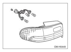
2. Remove the bulb holder from the rear combination light assembly by turning it counterclockwise.
