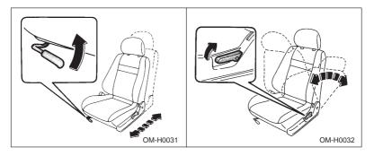
Pull the lever upward and slide the seat to the desired position. Then release the lever and move the seat back and forth to make sure that it is securely locked into place.
