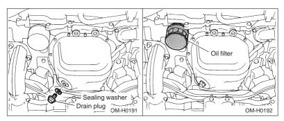
6. Remove the oil filter with an oil filter wrench.
