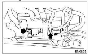
5) Remove spark plugs with the spark plug socket.
