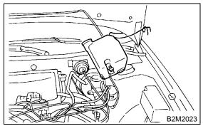
Disconnect connector from ignition coil.
