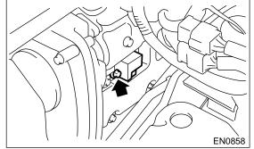
7) Remove spark plug with the spark plugs socket.
