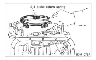
4) Position snap ring in transmission. Using ST, press the snap ring into place.
