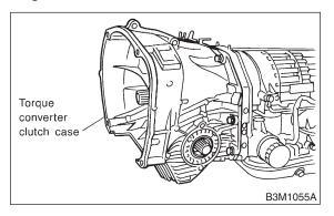
9) Remove the oil pump housing.
