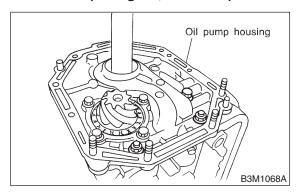
16) Apply proper amount of liquid gasket (THREE BOND Part No. 1215) to the entire torque converter clutch case mating surface.
