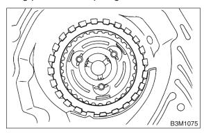
7) Install 2-4 brake oil seal to transmission case.
