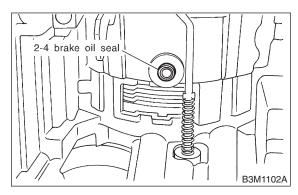
8) After all 2-4 brake component parts have been installed, blow in air intermittently and confirm the operation of the brake.
