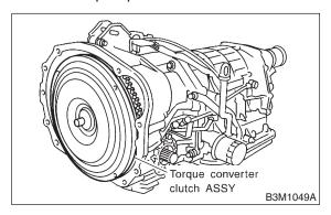
2) Remove the input shaft.
