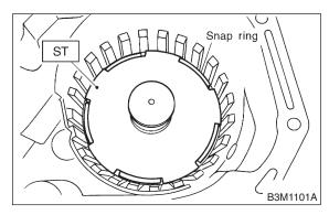
5) Install planetary gear and low clutch assembly to transmission case.
