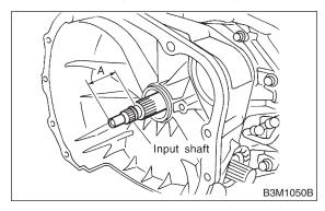
23) Install the torque converter clutch assembly.
