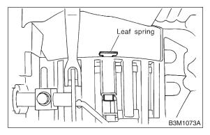
13) Take out retaining plate, drive plate and driven plate of 2-4 brake.
