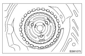
14) Take out the thrust needle bearing, planetary gear assembly and the low clutch assembly.
