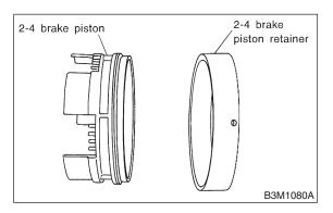
2) Install 2-4 brake piston and retainer to transmission case.
