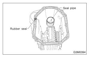
17) Install the torque converter clutch case assembly to the transmission case assembly, and secure with six bolts and four nuts.
