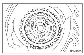
12) Install front sun gear and thrust needle bearing.
