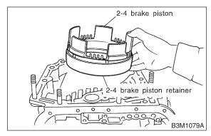
18) Separate 2-4 brake piston and piston retainer.
