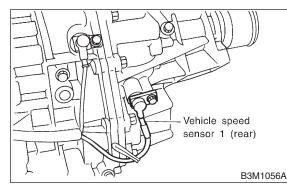
2) Separate transmission case and extension case sections.
