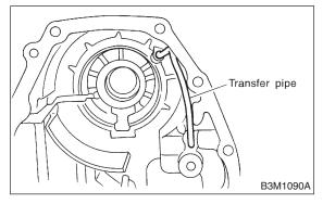
4) Install the transfer clutch assembly to the case.
