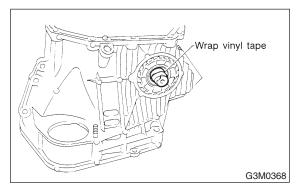
4) Install the oil seal and outer race (taper roller bearing) to the differential side retainer. Then screw in the retainer and the O-ring after coating the threads with oil.
