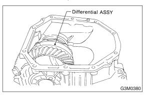
2) Install the circlip to the axle shaft, insert the shaft into the differential assembly, and tap it into position with a plastic hammer.
