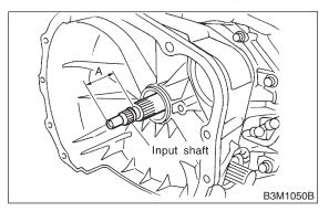
16) Install the torque converter clutch assembly.
