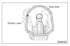
9) Apply proper amount of liquid gasket (THREE BOND Part No. 1215) to the entire torque converter clutch case mating surface.
