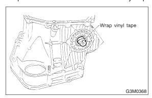
10) Remove the differential side retainer with ST.
