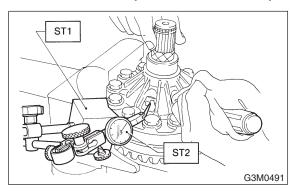
5) Using ST, install taper roller bearing. ST 398487700 DRIFT
