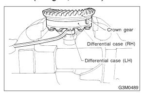
4) Measurement of backlash (Selection of washer) Measure the gear backlash with ST1 and ST2, and insert ST2 through the access window of the case.
