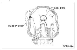
10) Install the torque converter clutch case assembly to the transmission case assembly, and secure with six bolts and four nuts.
