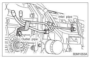
4) Install oil charger pipe with O-ring. <Ref. to AT-24 INSTALLATION, Oil Charger Pipe.>
