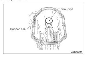
8) Install the torque converter clutch case assembly to the transmission case assembly, and secure with six bolts and four nuts.
