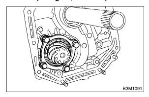
3) Install two oil seals to the oil seal retainer with ST.
