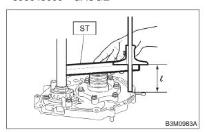
3) Calculation of total end play Select suitable bearing race from among those listed in this table so that clearance C is in the 0.25 to 0.55 mm (0.0098 to 0.0217 in) range.
