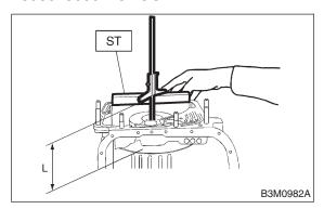
2) Using ST, measure the distance from the oil pump housing mating surface to the top surface of the oil pump cover with thrust needle bearing. ST 398643600 GAUGE
