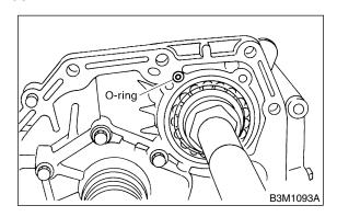
5) Install the oil seal retainer taking care not to damage the oil seal lips. Then secure with three bolts.
