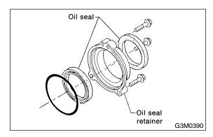
4) Attach the O-ring to the oil seal retainer with vaseline. Install the seal to the oil pump housing bore.
