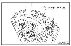
15) Remove the oil seal retainer. Also remove the O-ring and oil seal (air breather).
