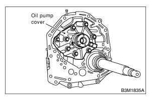
Install the oil seal retainer and seal rings. After adjusting the drive pinion backlash and tooth contact.
