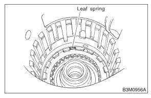
7) Install 2-4 brake piston, retainer and return spring to transmission case. <Ref. to AT-90 INSTALLATION, 2-4 Brake.>
