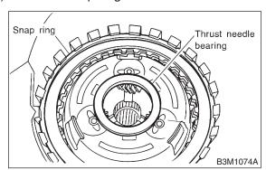
20) Take out retaining plate, drive plate and driven plate of 2-4 brake.
