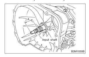
33) Install the torque converter clutch assembly. <Ref. to AT-30 INSTALLATION, Torque Converter Clutch Assembly.>
