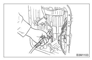
13) Measure the clearance between the retaining plate and the snap ring.
