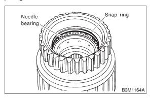
2) Install the one-way clutch, one-way clutch inner race and plate, and secure with the snap ring.
