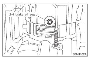
12) After all 2-4 brake component parts have been installed, blow in air intermittently and confirm the operation of the brake.
