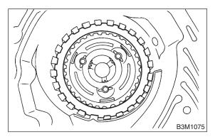
16) Install front sun gear and thrust needle bearing.
