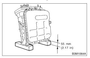
15) Remove the oil pump housing.
