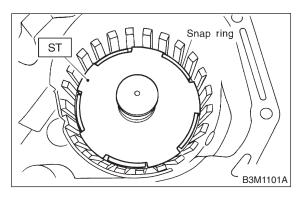
9) Install planetary gear and low clutch assembly to transmission case.
