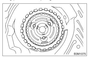
11) Install 2-4 brake oil seal to transmission case.
