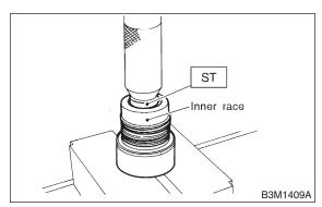
2) Install two seal rings to one-way clutch inner race.
