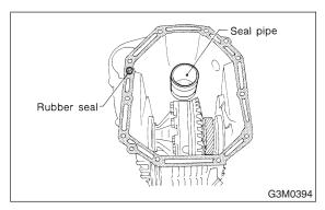
23) Install the torque converter clutch case assembly to the transmission case assembly, and secure with six bolts and four nuts.
