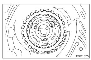
21) Take out the thrust needle bearing, planetary gear assembly and the low clutch assembly. <Ref. to AT-80 REMOVAL, Planetary Gear and Low Clutch.>
