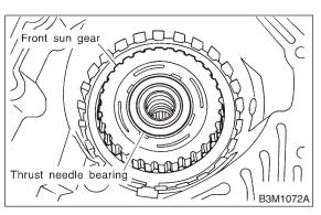
17) Install the high clutch hub and thrust needle bearing.
