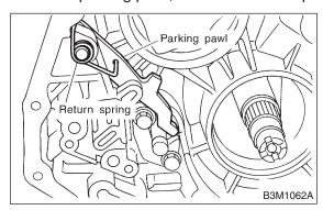
2) Install the extension case to the transmission case. <Ref. to AT-31 INSTALLATION, Extension Case.>
