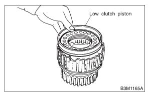
3) Install spring retainer to low clutch piston.
