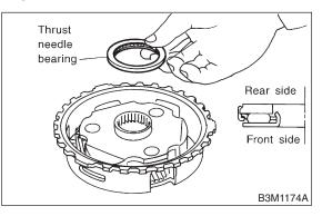
17) Install front planetary carrier to low clutch drum.
