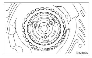
16) Take out the thrust needle bearing, planetary gear assembly and the low clutch assembly.
