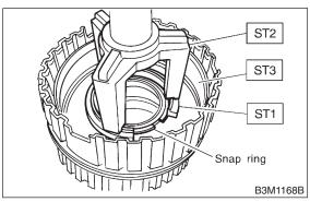
6) Install the dish plate, driven plates, drive plates, and retaining plate, and secure with the snap ring.
