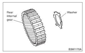
10) Install rear internal gear.
