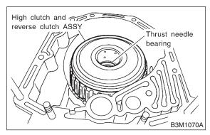
7) Install the high clutch hub and thrust needle bearing.
