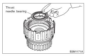
12) Install washer to rear planetary carrier.
