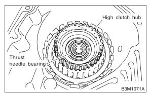
8) Adjust total end play. <Ref. to AT-79</li>ADJUSTMENT, High Clutch and Reverse Clutch.>9) Remove four seal rings.
