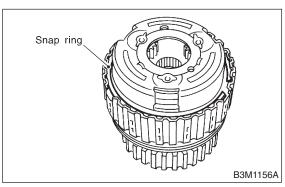
2) Take out front planetary carrier and thrust needle bearing from low clutch drum.
