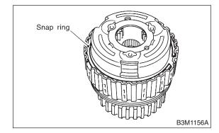
19) Install the needle bearing, and secure with the snap ring.
