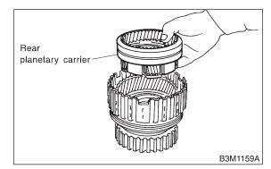
14) Install thrust needle bearing to rear planetary carrier.
