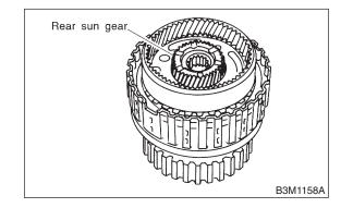
4) Take out rear planetary carrier, washer and thrust needle bearing.
