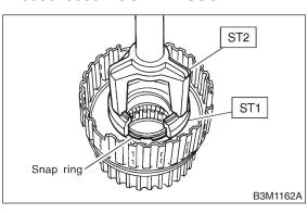
8) Install the one-way clutch inner race to the low clutch drum, and apply compressed air to remove the low clutch piston.
