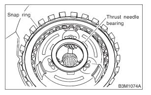
15) Take out retaining plate, drive plate and driven plate of 2-4 brake.
