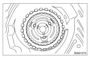
5) Install front sun gear and thrust needle bearing.<Ref. to AT-90 INSTALLATION, 2-4 Brake.>6) Install the high clutch assembly.
