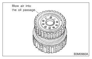
8) Checking low clutch clearance
