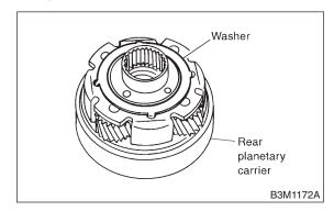
13) Install rear planetary carrier to low clutch drum.
