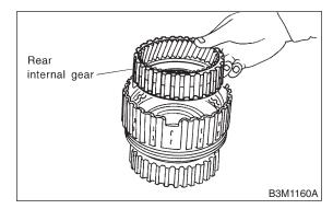
6) Remove the snap ring from the low clutch drum.
