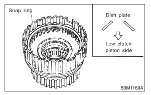
7) Check the low clutch for operation.
