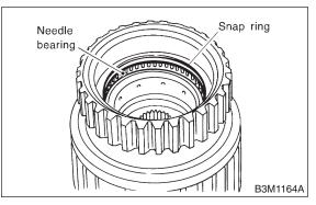
20) Install the one-way clutch, one-way clutch inner race and plate, and secure with the snap ring.
