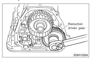
3) Using the ST1 and ST2, extract the reduction driven gear.
