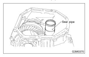
9) Install the rubber seal to the torque converter clutch case.
