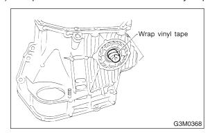
11) Remove the differential side retainer with ST.
