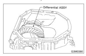
4) Install the circlip to the axle shaft, insert the shaft into the differential assembly, and tap it into position with a plastic hammer.
