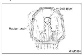
11) Install the torque converter clutch case assembly to the transmission case assembly, and secure with six bolts and four nuts.
