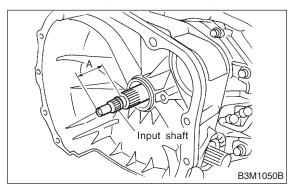
18) Install the torque converter clutch assembly. <Ref. to AT-30 INSTALLATION, Totque Converter Assembly.>
