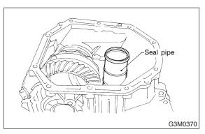
14) Remove the oil seal from torque converter clutch case.
