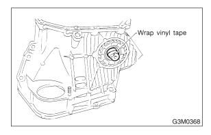
6) Install the oil seal and outer race (taper roller bearing) to the differential side retainer. Then screw in the retainer and the O-ring after coating the threads with oil.
