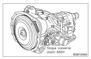
2) Remove the input shaft.
