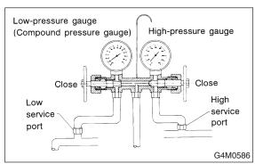
5) Connect the center hose to the refrigerant recovery system.
