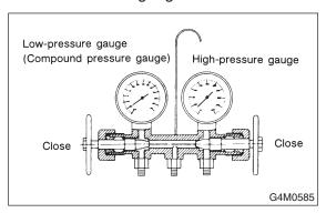
4) Install the low-/high-pressure hoses to the service ports on the low-/high-pressure sides of the vehicle respectively.
