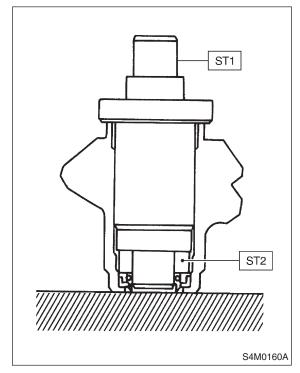
4) Using ST and press, install special bearing in valve housing.
