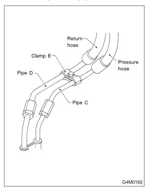
5) Disconnect pipe C from pipe (on the gearbox side).
