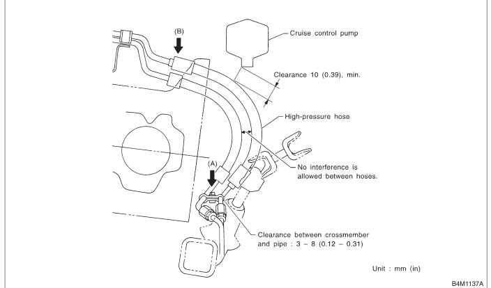
11) Finally check clearance between pipes and/or hoses, as shown.
