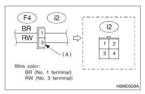
• In wiring diagram, connectors which have no terminal number refer to one-pole types. Sketches of these connectors are omitted intentionally.
