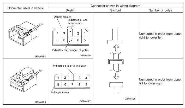
• When one set of connectors is viewed from the front side, the pole numbers of one connector are symmetrical to those of the other. When these two connectors are connected as a unit, the poles which have the same number are joined.
