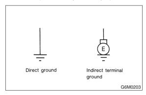
• The ground points shown in the wiring diagram refer to the following:
