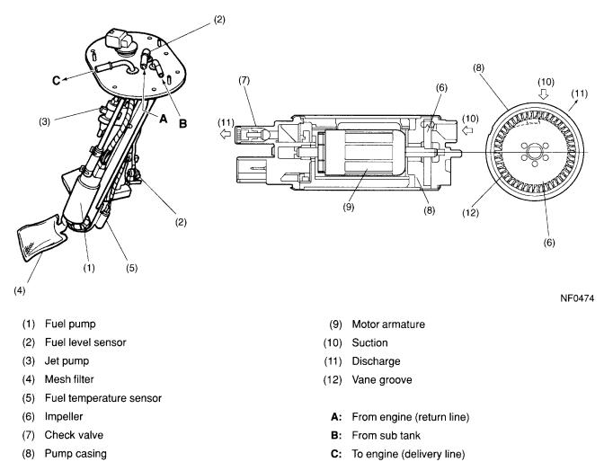
• When the ignition switch is turned ON, fuel pump relay is activated. Then the motor operates to rotate the impeller.
