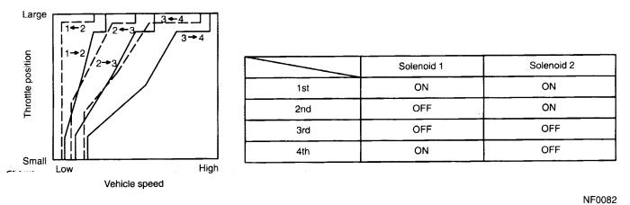
• The TCM activates both solenoids 1 and 2 in response to throttle and vehicle speed signals.
