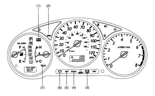
(1) CHECK ENGINE warning light This light illuminates when a fault occurs in the MFI (Multiple point Fuel Injection) system.
