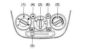
(1) Air flow control dial: This switch allows selecting any of the five air flow modes.
