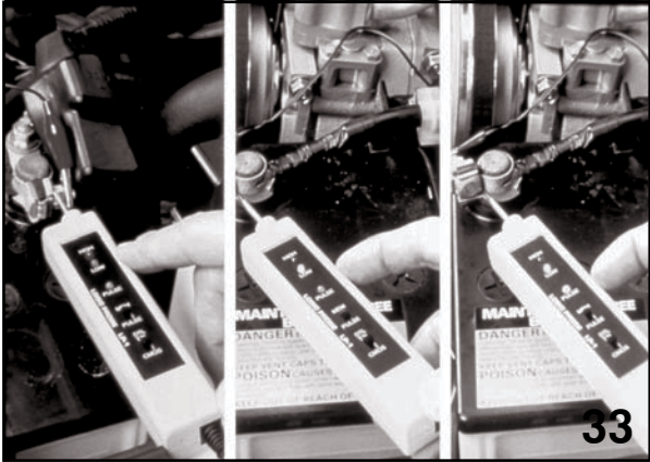
Digital logic probe (DLP)
