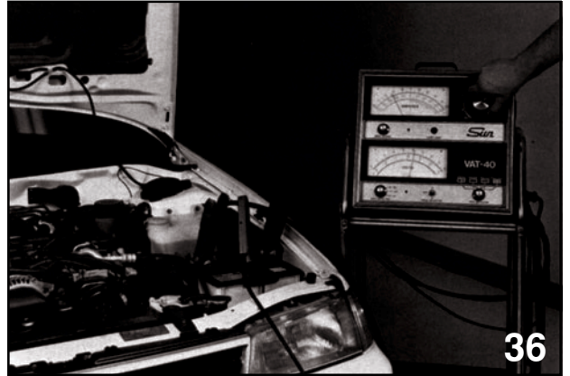
Battery performance test
