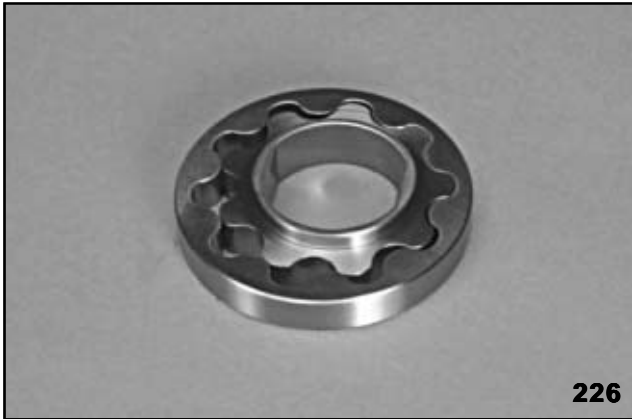
Pump Gears (Back Side)
