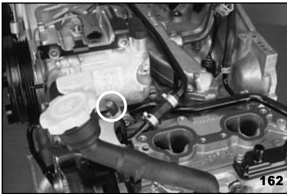
Factory Coolant Pipe Plug
