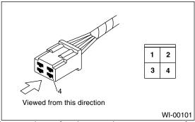
• The number of poles or pins, presence of a lock, and pin number of each terminal are indicated in the sketch of each connector. In the sketch, the highest pole number refers to the number of poles which connector has. For example, the sketch of connector shown in the figure indicates the connector has 9 poles.
