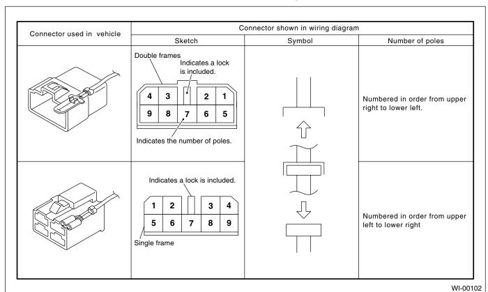
• When one set of connectors is viewed from the front side, the pole numbers of one connector are symmetrical to those of other. When these two connectors are connected as a unit, the poles which have the same number are joined.
