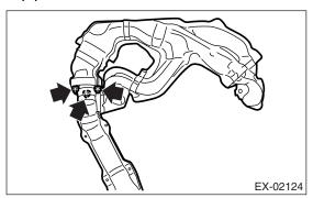
10) Remove the front oxygen (A/F) sensor and the rear oxygen sensor. <Ref. to FU(H4SO)-36, RE-MOVAL, Front Oxygen (A/F) Sensor.> <Ref. to FU(H4SO)-37, REMOVAL, Rear Oxygen Sensor.>
