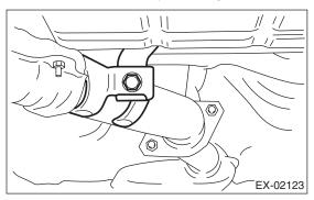
8) Remove the front and center exhaust pipe assembly from vehicle.
