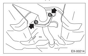
2) Separate the rear exhaust pipe from muffler.
