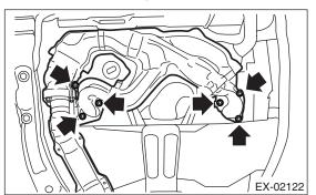
7) Remove the bolt which installs the front and center exhaust pipe assembly to hanger bracket.
