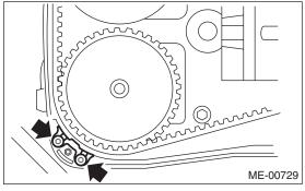
11) Turn the crankshaft and align the alignment marks on crankshaft, and left and right cam sprockets with notches of belt cover and cylinder block. Use the ST to turn crankshaft.
