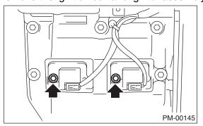
Spark Plug Periodic MAINTENANCE SERVICES 5) Remove the spark plug with a spark plug socket.
