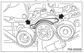
11) Turn the crankshaft and align the alignment marks on crankshaft, and left and right cam sprockets with notches of belt cover and cylinder block.
