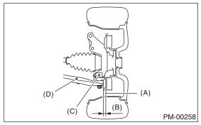
3) Grasp the transverse link and move it up and down. Relative movement (A) between the housing (D) and transverse link (C) boss indicates ball joint (B) may be excessively worn.
