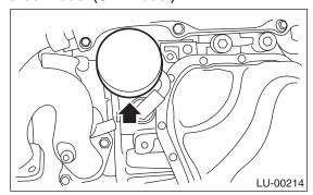
3) Clean the oil filter installation surface on cylinder block or oil cooler.
