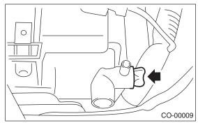
5) For quick draining, open the radiator cap.
