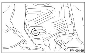
3) Replace the gasket with a new part and tighten the differential oil drain plug to the specified torque using the TORX® bit T70.
