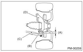
4) If the relative movement is observed in the preceding two steps, remove and inspect the ball joint. If the free play exceeds the standard, replace the ball joint. <Ref. to FS-16, Front Ball Joint.>
