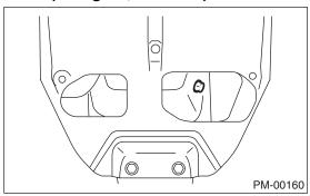
5) Using engine oil of proper quality and viscosity, fill engine oil through the oil filler duct to the upper level on level gauge. Place the vehicle on a level surface when checking oil level.
