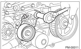
16) Install in the reverse order of removal. <Ref. to MÉ(H4SO)-44, INSTALLATION, Timing Belt.>
