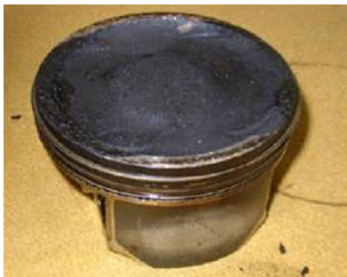
Ring Land Damage from Detonation
