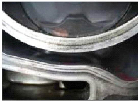
After cleaning oil sealing portion (block)
