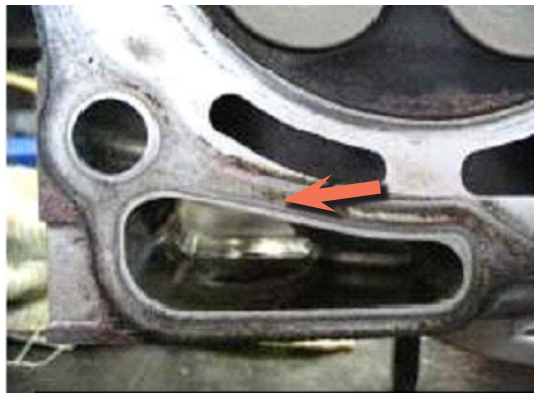
Rubber coating residue on oil sealing portion
