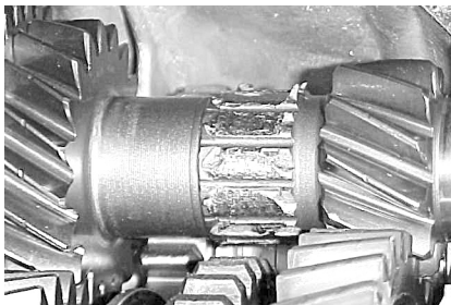
Reverse Gear Teeth Stripped
