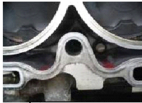
After cleaning coolant sealing portion (block)
