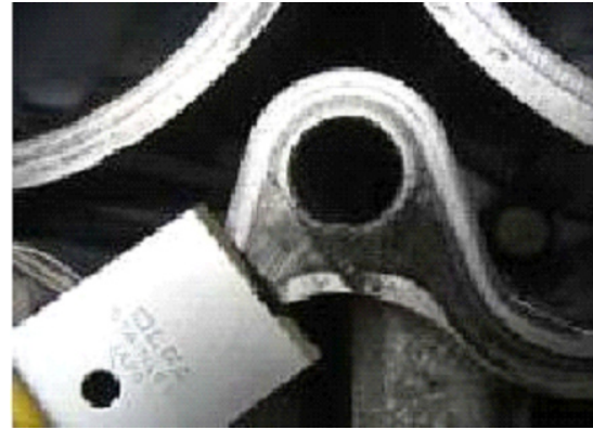
Rubber coating being removed
