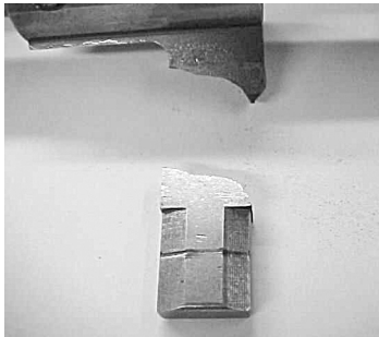
6-Speed 1-2 Shift Interlock Arm Broken
