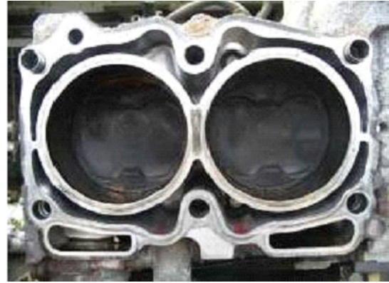
Finished cleaning (block)
