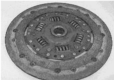
Over Heated Clutch Disc
