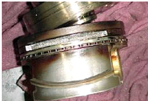
Ring Land Broken from Over Boosting
