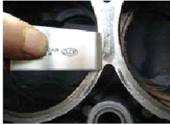
Carbon deposits being removed
