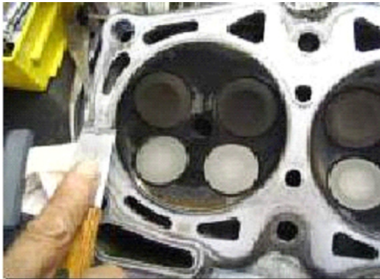
Rubber coating being removed
