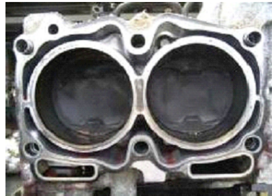
Cylinder Block after Head Removal
