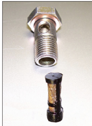
Banjo bolt and Mesh Screen (note direction of screen)
