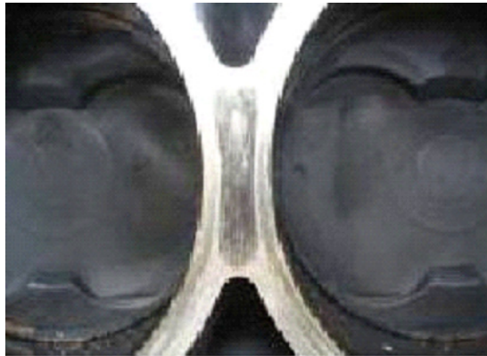
After cleaning bore sealing portion (block)
