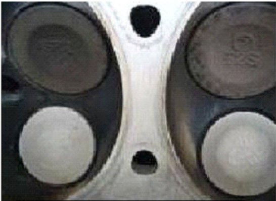
After cleaning bore sealing portion (head)
