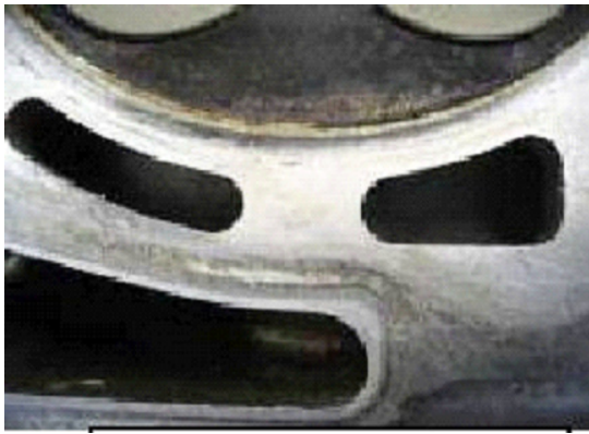
After cleaning oil sealing portion (head)
