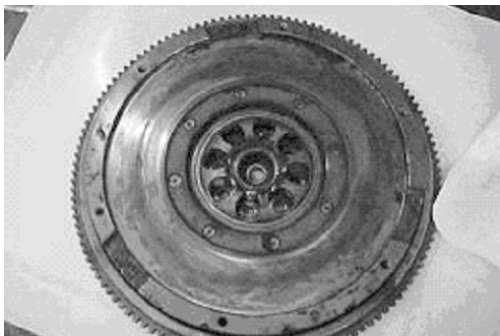
Over Heated Flywheel
