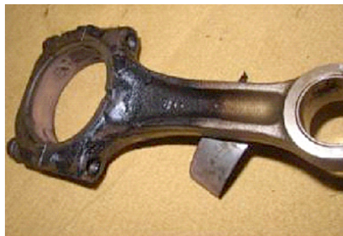
Rod Bearing Spun from Lack of Oil
