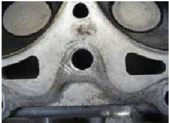
After cleaning coolant sealing portion (head)
