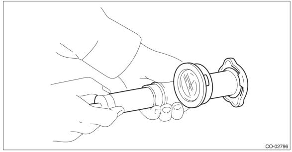
3) Increase pressure until the radiator cap tester gauge needle stops. Radiator cap is functioning properly if it holds the service limit pressure for 5 — 6 seconds. Replace the radiator cap if its valve opens at less than the service limit.
