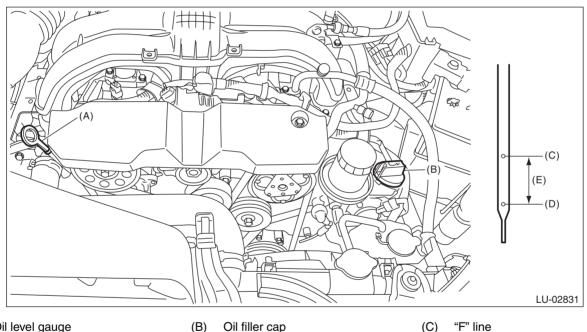
(A) Oil level gauge Oil filler cap
