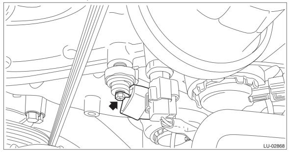
4) Remove the oil pressure switch.
