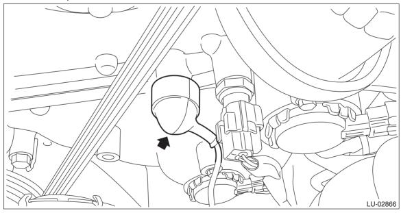
5) Connect the battery ground terminal.
