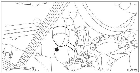
3) Disconnect the terminal from oil pressure switch.
