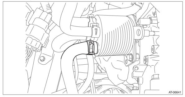
11) Remove the electric power steering harness from the clip, and remove the engine coolant inlet hose from the engine coolant pipe.
