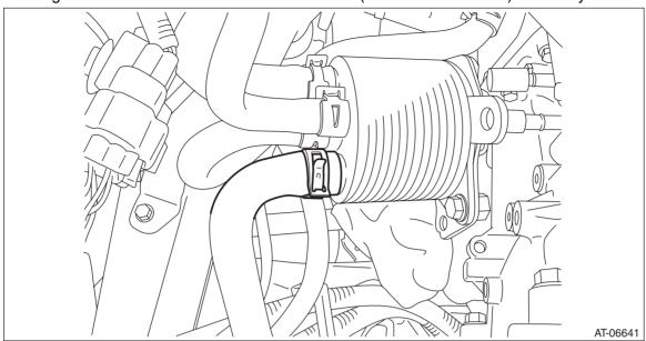
3) Install the CVTF inlet hose and CVTF outlet hose to transmission.
