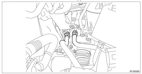
10) Disconnect the engine coolant inlet hose from the CVTF cooler (with warmer feature) assembly.
