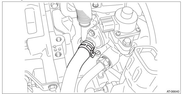
6) Install the engine hanger rear.
