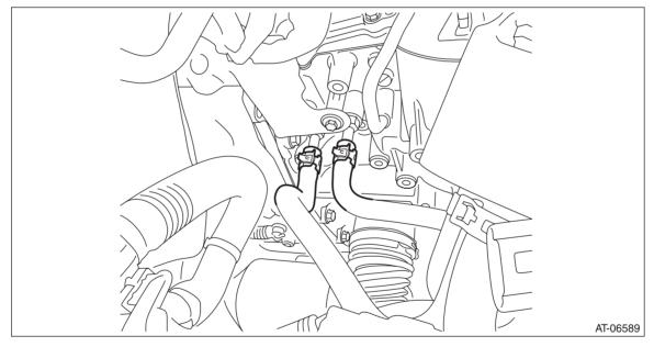
4) Install the CVTF cooler (with warmer feature) to the transmission.
