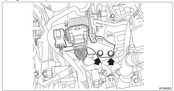
7) Connect the EGR control valve harness connector, throttle position sensor harness connector and manifold pressure sensor harness connector.
