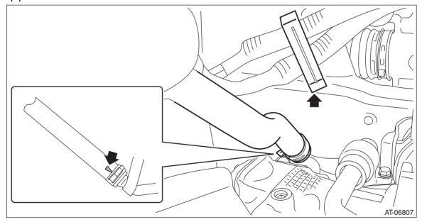
2) Install the engine coolant inlet hose to the CVTF cooler (with warmer feature) assembly.
