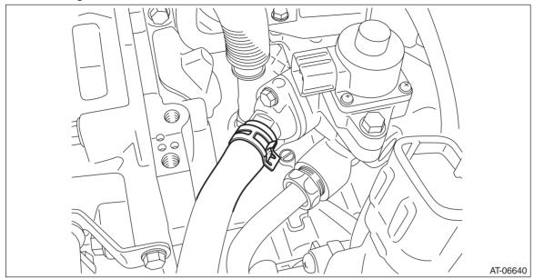
8) Remove the CVTF cooler (with warmer feature) from the transmission.
