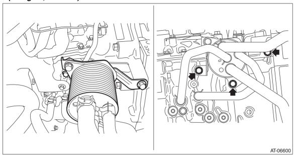
5) Connect the engine coolant outlet hose.
