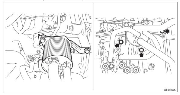
9) Remove the CVTF inlet hose and outlet hose from the pipe on the transmission side.
