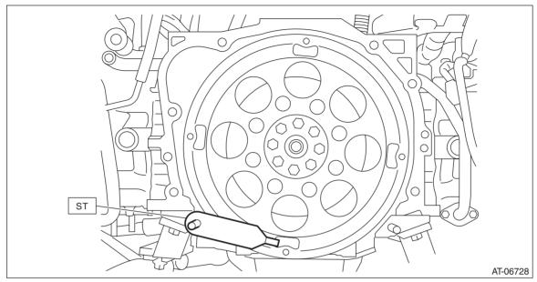
3) Remove the drive plate and reinforcement drive plate.
