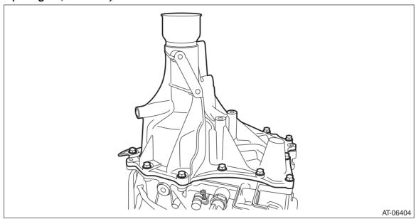
9) Install the transmission assembly. <Ref. to CVT-67, INSTALLATION, Automatic Transmission Assembly.>
