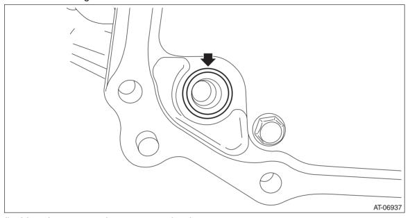
7) Apply liquid gasket to extension case seamlessly.
