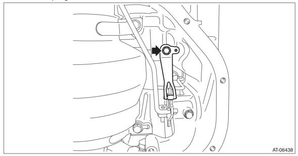
6) Remove the manual plate from the shifter arm shaft, and remove the shift connecting rod of the manual valve.
