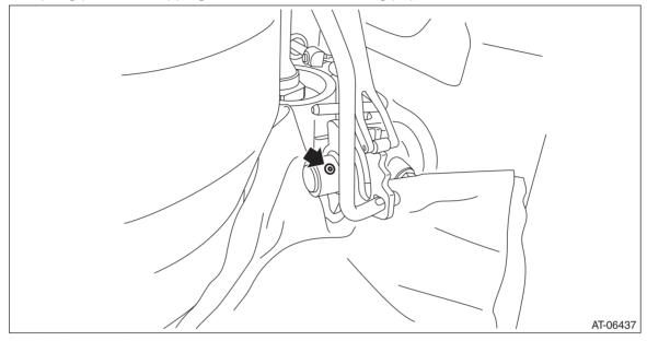
5) Remove the detent spring.
