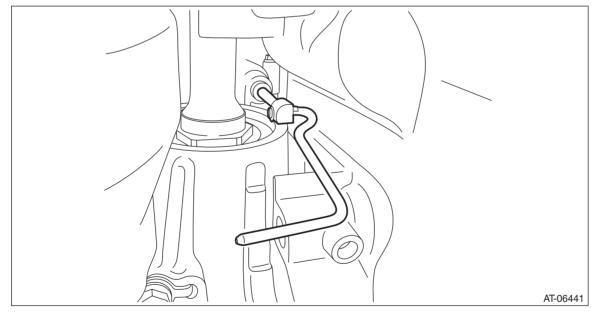
4) Install the shifter arm shaft and bolt.
