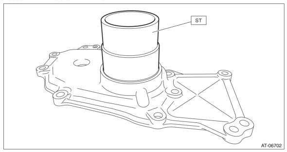
3) Install the drive sprocket.
