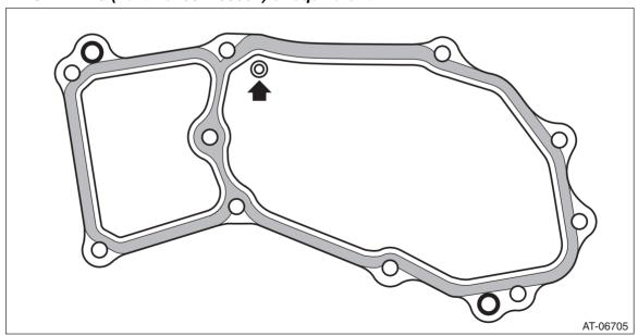
9) Install the oil pump chain cover.
