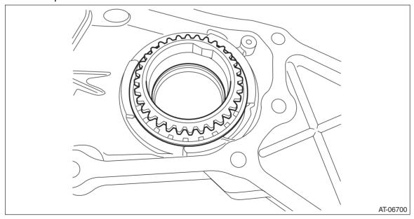
4) Install the snap ring so that its cutout portion is securely fitted into the snap ring groove of the oil pump chain cover.
