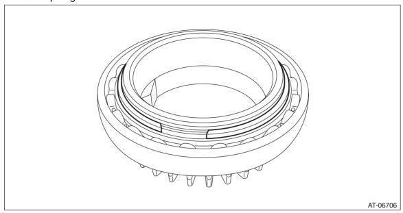
2) Remove the ball bearing using ST. ST1 498077600 REMOVER **INSTALLER** ST2 399513600
