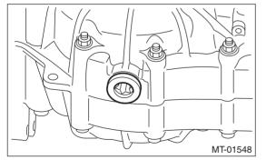
5) Remove the center exhaust pipe. <Ref. to EX(H4DO)-14, REMOVAL, Center Exhaust Pipe.> 6) Separate the front drive shaft from the transmission. <Ref. to DS-57, REMOVAL, Front Drive Shaft.> 7) Remove the differential side retainer oil seal.
