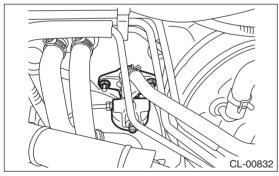
8) Remove the bolts and nuts which secure the brake pedal and clutch pedal, and remove the pedal assembly.
