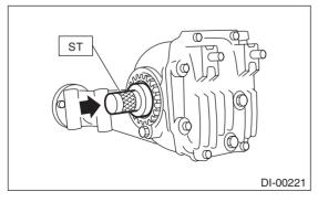
4) Install the rear differential. <Ref. to DI-24, IN-STALLATION, Rear Differential (T-type).> <Ref. to DI-41, INSTALLATION, Rear Differential (VAtype).>
