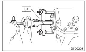
3) Using the ST, install the oil seal.
