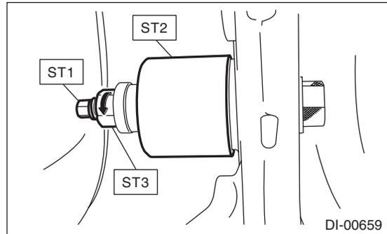
8) Hold the ST1 with a tool to prevent it from rotating, and screw in the ST2 to remove the rear differential mount bushing.
