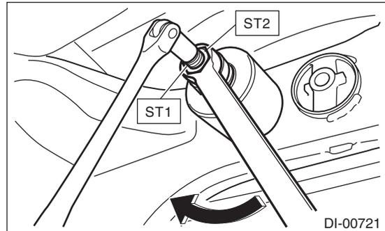
14) Make sure that the rear differential mount bushing is inserted to the front end of sub frame cylinder.
