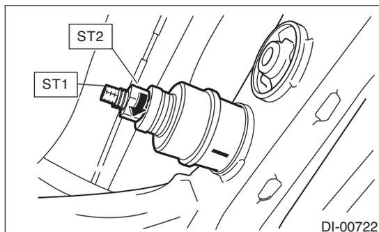
13) Screw in the ST2 while holding the ST1 with a tool to prevent it from rotating, and press-fit the rear differential mount bushing to the front end of sub frame cylinder.
