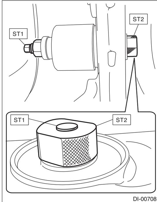
7) Hold the ST1 to prevent it from rotating, and screw in the ST3 by hand till there is no loose fit on the ST2.
