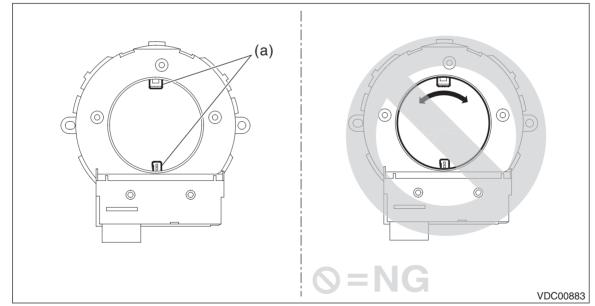
(2) Align the center of steering roll connector. < Ref. to AB-107, INSTALLATION, Roll Connector.>
