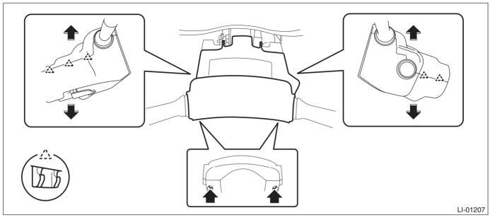
7) Remove the steering roll connector.
