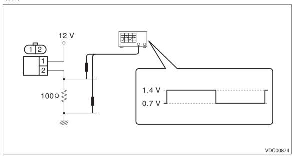
5) Replace the ABS wheel speed sensor if the inspection result is not within the standard value.
