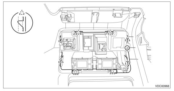
3) Release the claws and remove the VDC OFF switch.
