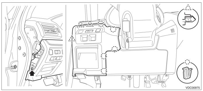
2) Remove the screws and release the claws, then detach the cover.
