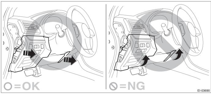
(1) Remove the clips, and remove the cover - instrument panel side LH.
